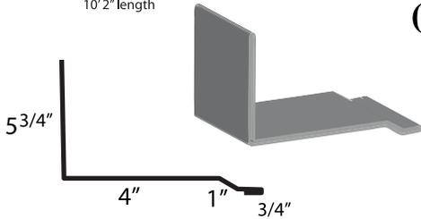
**DC Sidewall Flashing (Transition Flashing)** <sup>15</sup> \*
